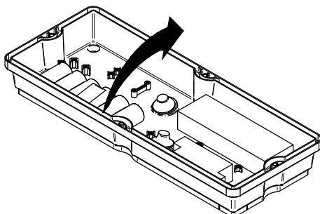
**6 | Emergency module disassembly**
