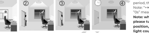
1. With ambient light more than daylight threshold, the lamp does not switch on when someone enters the room.
