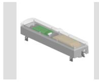
Dedicated emergency kit made in grey PC (RAL 7035) for Smart[3] through wiring version. Equipped with Ni-Mh batteries for 3h autonomy. Can be fitted on the unit itself using fixing springs or mounted on the wall/ceiling, using 4mm screws.
