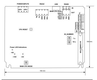
Note! Both 24VDC inputs must be connected.
