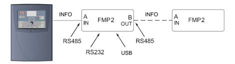
**Note!** The maximum number of DAP2, FMP2, REPX, REPX-OB, MCOX, MCOX-OB, ZLPX, ZLPX-IC units connected to one FX-panel is 16.
