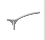
Single pole head bracket in hot galvanised steel tubing, 3 or 4mm thick, painted with polyester powder. Supplied with three M8 stainless steel lockscrews for fixing on poles of 60mm diameter.
