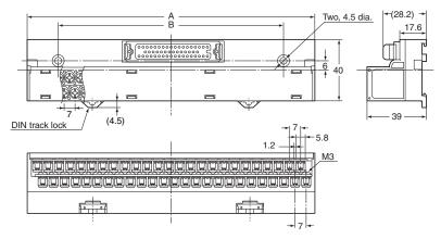
Note: There is only one DIN Track lock located in the center of the Connector for a 20-pole Unit.
