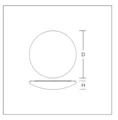
Decorative round surface-mounted luminaire. For escape route illumination. Base: metal, powder-coated. Diffuser made of non-yellowing plastic (PMMA), opal. Diffuser fastening: patented push system. Suitable for Ceiling mounting, Wall (surface). Electronic ballast included. Self-contained system with automatic self-test.
