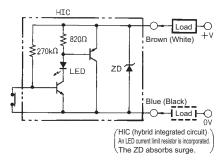
Note: The load may be connected to either the +V or 0 V terminal.
