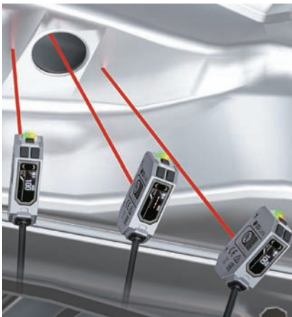
Parts identification using hole positions
