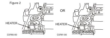
4. Connect the heater power supply wires as shown in Figure 3. If adding the heater kit to an existing installation, insure that the power supply connected to the beam detector is adequately rated for the additional power consumption of the heater.
