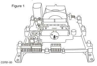
3. Plug the connector into pin-header labeled HEATER on the transmitter/ receiver PCB as shown in Figure 2. Pin orientation does not matter. Please insure that the connector is installed properly on all three pins, or the heater will not work.
