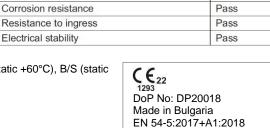
EN 54-5:2017+A1:2018 EN 54-17:2005/AC:2007 Detector Class: A1/R (rate of rise +58°C), A2/S (static +60°C), B/S (static +75°C)
