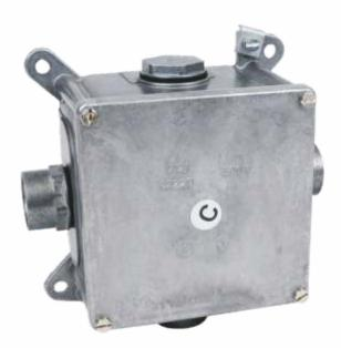
product description: designed for distribution system with voltage 500 V and with maximum current 16 A boxes for piping with steel threaded or metal flexible pipes three glands and one plug evenly distributed on the sides of the box or installation in TNC networks to install on materials with fire classes E or F, use thermally insulating pad dimension: 120x120x76 mm
