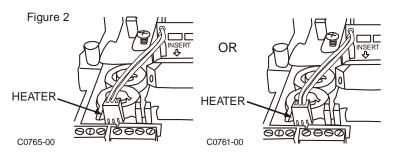
4. Connect the heater power supply wires as shown in Figure 3. If adding the heater kit to an existing installation, ensure that the power supply connected to the beam detector is adequately rated for the additional power consumption of the heater.
