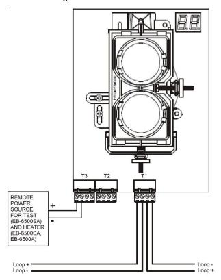
5. Align/realign beam smoke detector. Refer to the installation manual provided with the beam smoke detector for alignment instructions.
