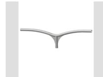
Double pole head bracket in hot galvanised steel tubing, 3 or 4mm thick, hot galvanised steel and painted with polyester powder. Supplied with three M8 stainless steel lockscrews for fixing on poles of 60mm diameter.
