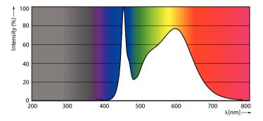
Spectral Power Distribution Colour - MAS LEDtube 1200mm HO 12.5W 840 т8
