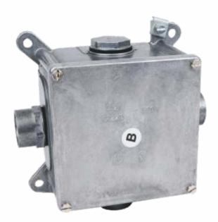
product description: designed for distribution system with voltage 500 V and with maximum current 16 A boxes for piping with steel threaded or metal flexible pipes three glands and one plug evenly distributed on the sides of the box fitted with a clamp for installation in TNS networks to install on materials with fire classes E or F, use thermally insulating pad dimension: 120x120x76 mm
