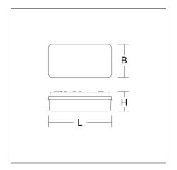
Luminaire for escape route identification. Base: plastic Diffuser: plastic, opal 4 plastic foils with escape route motifs included (ISO 7010). Suitable for Ceiling mounting, Wall (surface). Pendant luminaire also possible with accessories. Electronic ballast included. Self-contained system with automatic self-test and feedback to the RZB monitoring system MULTIDIGIT.
