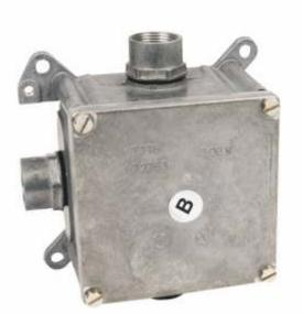
product description: designed for distribution system with voltage 500 V and with maximum current 16 A boxes for piping with steel threaded or metal flexible pipes three glands and one plug evenly distributed on the sides of the box fitted with a clamp for installation in TNS networks to install on materials with fire classes E or F, use thermally insulating pad dimension: 96x96x64 mm
