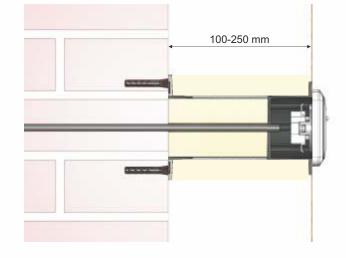
There is necessary to cut the carrier including inserted insulation before installation depending on layer thickness insulation.
