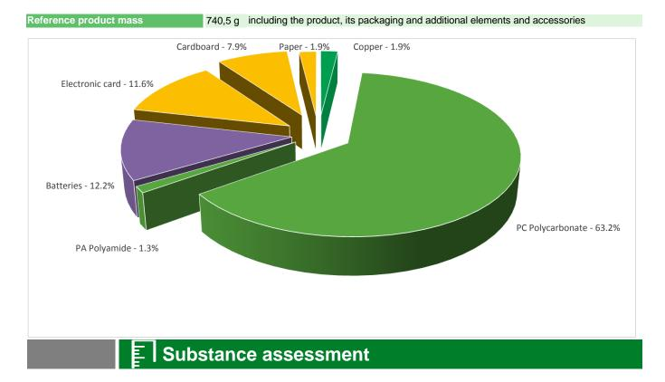
Products of this range are designed in conformity with the requirements of the RoHS directive (European Directive 2011/65/EU of 8 June 2011) and do not contain, or only contain in the authorised proportions, lead, mercury, cadmium, hexavalent chromium or flame retardants (polybrominated biphenyls - PBB, polybrominated diphenyl ethers - PBDE) as mentioned in the Directive
