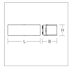
Luminaires for escape route identification Base: metal, powder-coated. Diffuser: plastic (polycarbonate), opal. 4 plastic foils with escape route motifs included (ISO 7010). Driver integrated. Suitable for connection to central battery systems.
