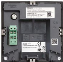
Connection with FDM121 display unit.
