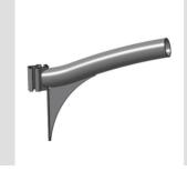
Bracket for fixing on poles of 60-75mm diameter, in hot galvanised steel tubing, 3mm thick, painted with polyester powder. Stainless steel screws and nuts.
