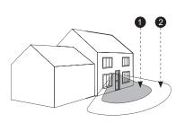
For optimum coverage recommended mounting height: 1m to 2.2m
