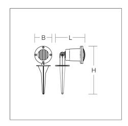
Garden spotlight with earth spike and protective grille for PAR16 mains-voltage reflector lamps. Housing and protective grill: die-cast aluminium, powder-coated. Safety glass, clear. Peg made of fiber reinforced plastic. With 3 m connection cable including safety plug (Schuko).
