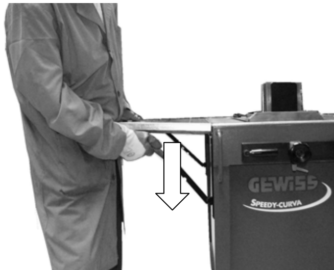
Fig. 3.11 – Supporting surfaces fastening system
