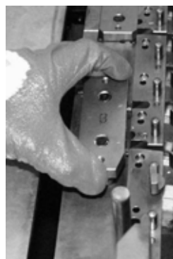
Fig. 4.51 – Positioning of second right fulcrum 3 in the arm with position X3 on the left
