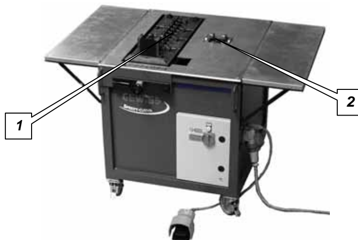
Fig. 5.1 – Location of the bending and cutting station.
