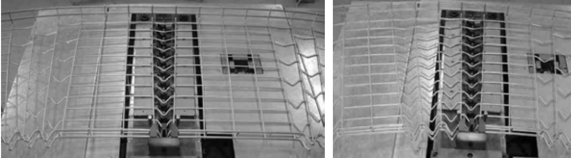
Fig. 4.78 – Bending of 4 left central sectors included among bends of alternate cut wires
