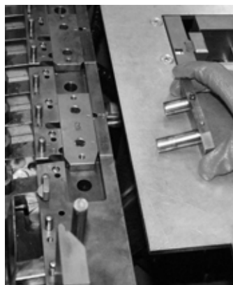
Fig. 4.48 – Positioning of first fulcrum 3 on the worktable
