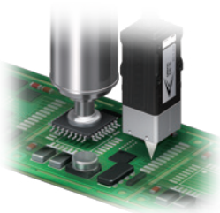
Z axis adjustment of chip mounter
