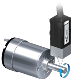
Eccentricity measurement of motors
