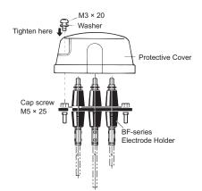
Note: The Protective Cover cannot be mounted on the BF-1.
