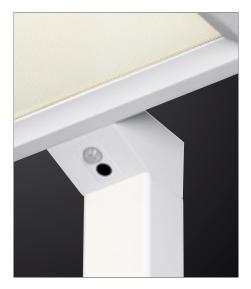
Daylight and motion sensor (PIR) reduces light output after 30 minutes without motion detection. After a further 30 minutes, the light automatically switches off.
